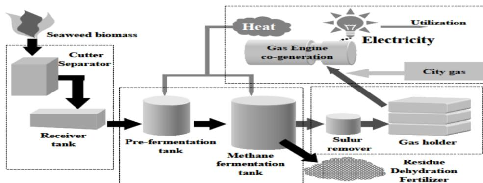
**Figure 2. Seaweed processing plant for production of methane and electricity (Matsui et al., 2006)**
