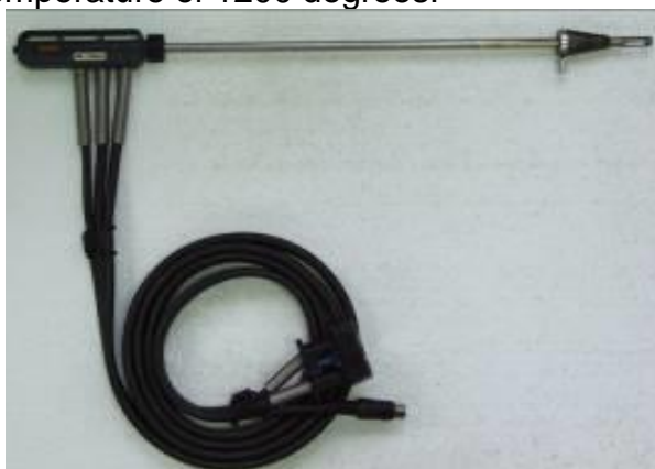
Figure 5 - The sampling probe for gas [8]
