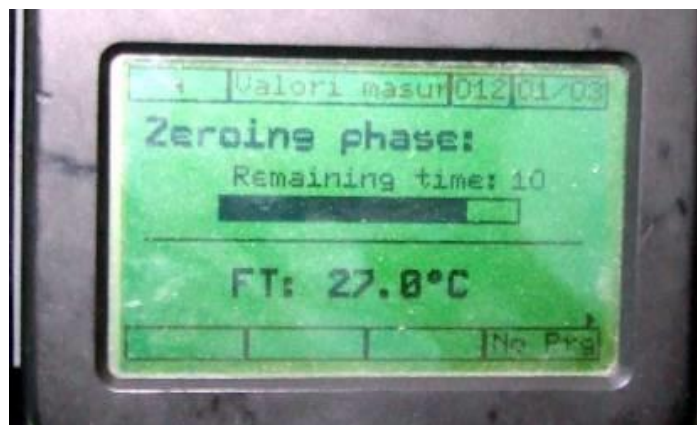
Figure 6 – Zero calibration for Testo 350 M/XL [8]
