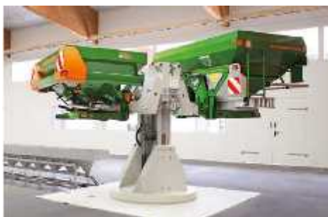
Fig. 15 - The test stand for experimental administering machines for mineral fertilizer firm Amazone [11]
