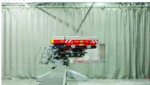
Fig. 14 - The test stand for experimental machines for administered mineral fertilizer firm Vicon [14]
