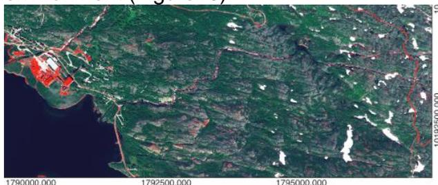
Figure 10: Mapping of mine tailings and ARD using WorldView-3 satellite imagery with spatial resolution of 2,5 m
