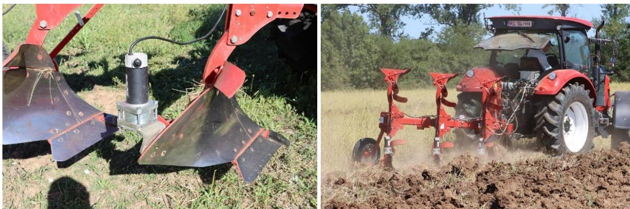
**Fig.1. – Mounting the electro-vibrators on each body of the reversible plough**
