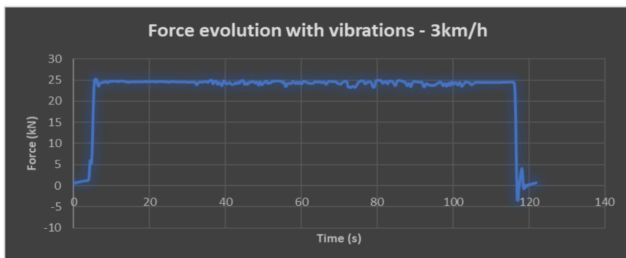
**Fig.3. – Graphical representation of the evolution of Traction Force - with the vibration systems activated**
