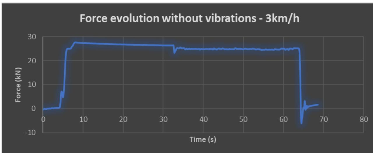
**Fig.2. – Graphical representation of the evolution of Traction Force - without activating the vibration systems**
