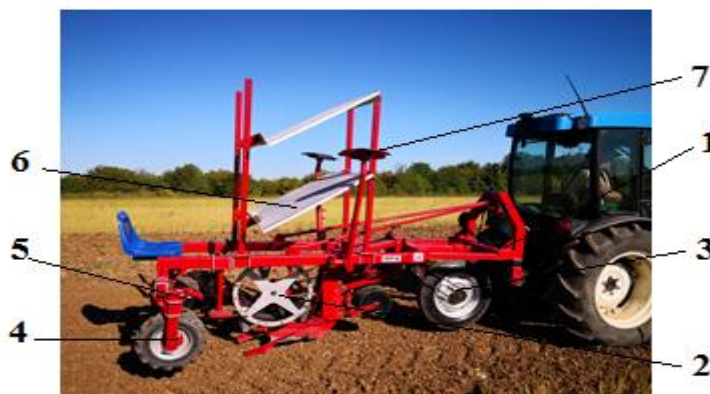
Fig.1 Machine for planting vegetable seedlings and herbs in a row, MPA symbol (**** INMA Bucharest, 2018)
