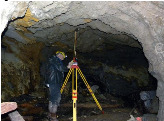
Figure 4: Wall station traversing: configuration of instrument
